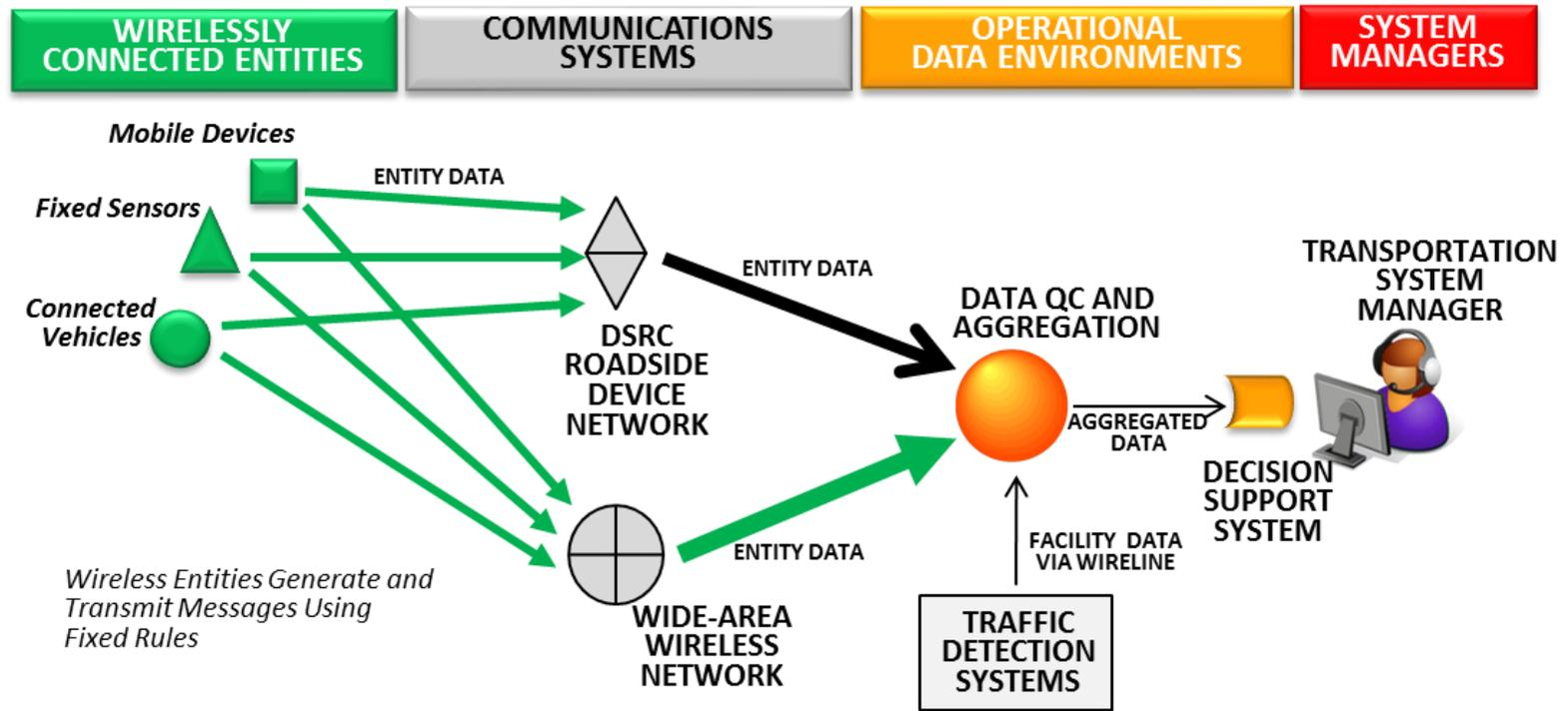
Figure 1-2: Unconstrained Data Capture (Source: Noblis, 2014)
